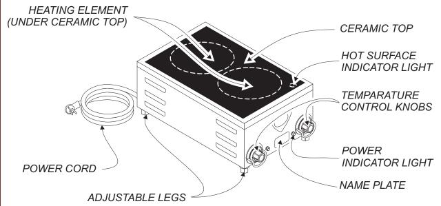
Ceramic Top Provides smooth, low maintenance heating surface
